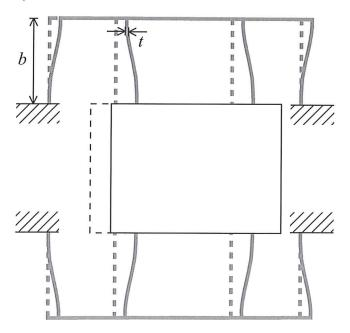
a. First determine the stiffness  $k_1 := F/U$  of a *single* leaf spring against a sideway displacement U, see figure below (this can be done either by solving the differential beam equation (3.49) plus boundary conditions or by application of the vergeet-me-nietjes of Fig. 3.6).
