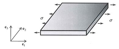
Assume a uniaxial stress state (i.e. plane stress in both  $e_2$ - and  $e_3$ - directions). Determine the most likely slip plane(s) and slip direction(s), i.e., the one(s) where the resolved shear stress is maximum.
