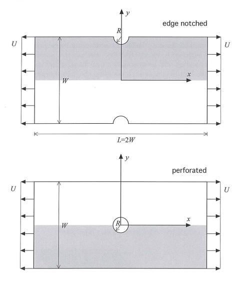
The total amount of material left is the same, and in fact the gray areas indicating symmetric halves are identical. Nevertheless, the two plates will respond to an applied end displacement U in different ways (even if they have the same uniform material properties). Apparently something in the entire set of governing equations is different; the question is: what?
